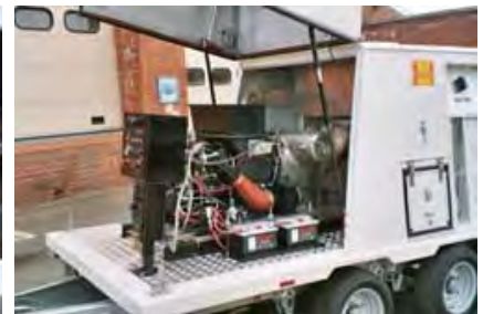
Mobile Air Start Unit, ATS 8084 with Garrett Turbine
