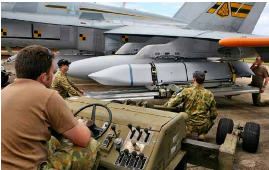
ARLU technicians load the JASSM on to the test Hornet at RAAF Base Williamtown during the trial. Photo: SGT Shane Gidall
