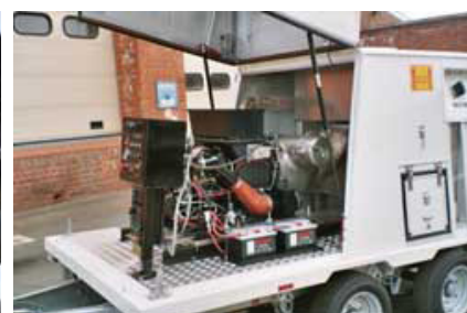
Mobile Air Start Unit, ATS 8084 with Garrett Turbine
