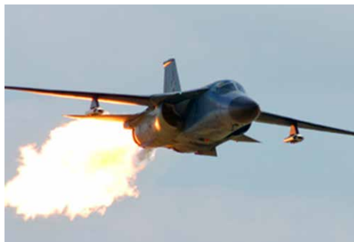
An F-111C carrying out a fuel 'dump and burn' at low level. Photo: RAAF
