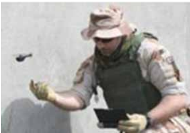
The Black Hornet: a nano UAS personal reconnaissance system. Photo: Prox Dynamics
