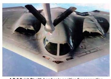
A B-2 Spirit Stealth bomber in position for connection to take on fuel. Photo: USAF
