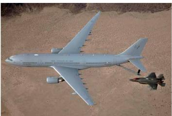
A RAAF KC-30A Multi-Role Tanker Transport makes contact with the receptacle of a USAF F-35A Joint Strike Fighter during boom refuelling trials in the United States. The F-35A is equipped with symmetrical external stores for this trial.
