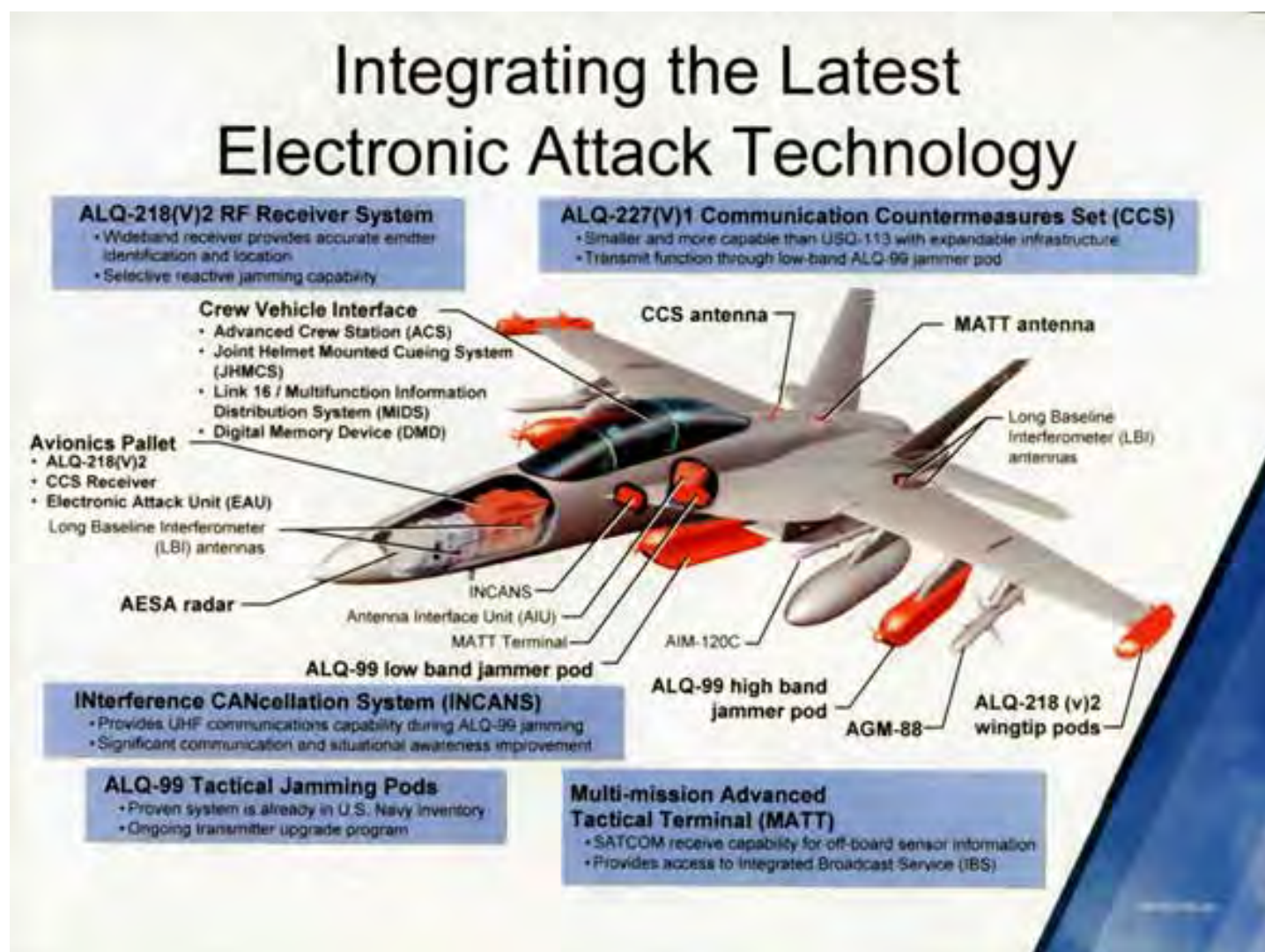
A cutaway diagram showing the key EW systems. Photo: Boeing/USN
