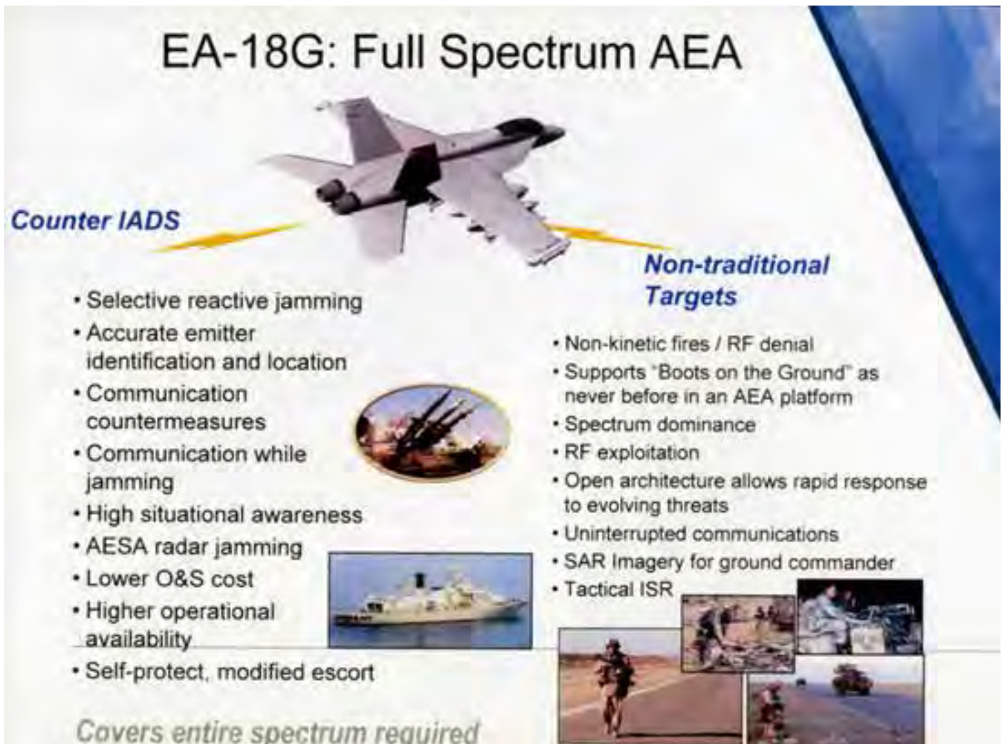
Diagram depicting the Full Spectrum Airborne Electronic Attack (AEA) provided by the EA-18G Growler Photo: Boeing/USN
