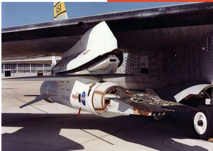
BELOW The X-43A hypersonic research vehicle and its modified Pegasus booster rocket mounted to NASA's NB-52B carrier aircraft at the Dryden Flight Research Center, Edwards, California. Photo: NASA.
