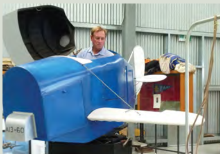
LEFT NAHC's Link Trainer, an early US flight simulator used for pilot training at Nhill and other RAAF stations.
