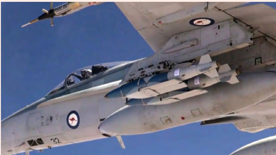
BELOW JDAM-ER is a high-precision glide bomb with a stand-off range of more than 70km.
