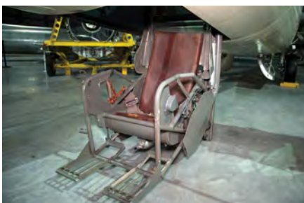
ABOVE Entry to the X-3 was via a rail-mounted, downward-firing ejection seat. Photo: NMUSAF.
