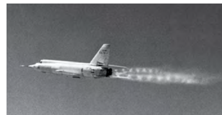
ABOVE X-2 with twin set of shock-diamonds characteristic of supersonic conditions in the exhaust plume from the two-chamber rocket engine. Photo: NASA.
