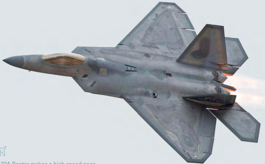
F-22A Raptor makes a high speed pass with engines in afterburn. Noteworthy are the closely-coupled stabilator and wings. Photo: LMSW.
