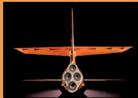
ABOVE The X-1's four rocket chamber nozzles.
