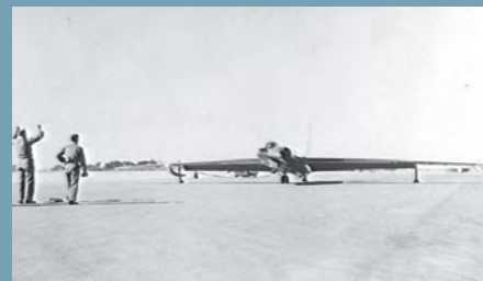
A U-2 modified for HASP flights – note the additional air scoops on the lower fuselage, and air valve in the nose.
